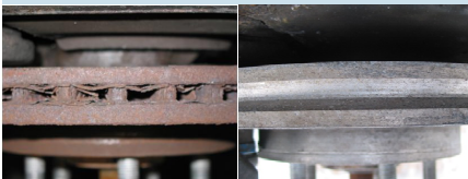
Cast iron and SCA rotors after 4 years service
